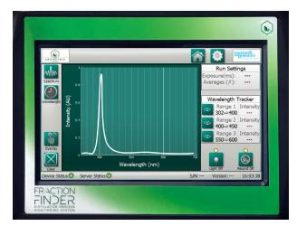
By monitoring the fluorescence in real-time immediately prior to the collection flask, manufacturers can use the tool to provide real-time insight into the efficiency and reliability of their distillation process.
