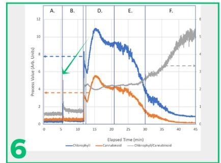
Observe no signal or noisy signal from reverberations during initial startup
