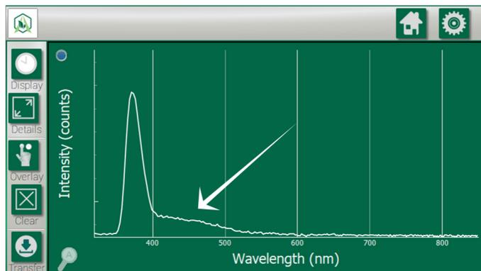
**Option B - Wavelength View:** This view will show that there is a big peak in the value of the wavelength plot. An example plot is shown below. The Wavelength View is recommended to identify when the distillation is transferring from Heads to Main Body.
