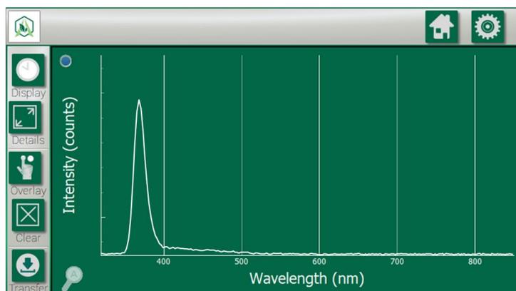
**What it does:** This is an instantaneous representation of the current spectral state. It displays the current background/ambient light corrected spectral measurement.
