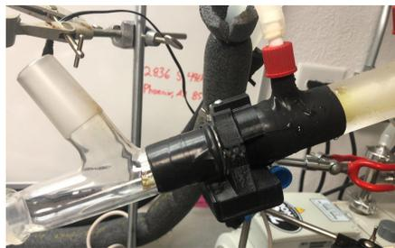
3. Insert the **sensor cable** into the back of the **sensor**.
