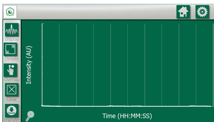
**What it does:** Displays and tracks the interpreted values from your measurement. This plot reduces the raw data and shows you the “highlights” of the run. This view is especially useful for tracking particular chemical oddities that occur at specific wavelengths.
