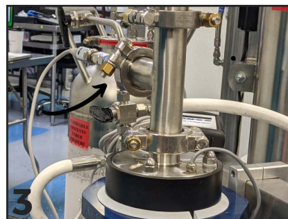
3 On the top-end, connect a second 1.5" Sanitary Flange to Hose Adapter (or equivalent) for outgoing flow.
