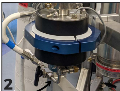
2 On the bottom-end of Extraction Housing, connect a 1.5" Sanitary Flange to Hose Adapter (or NPT or another connection) for incoming flow.
