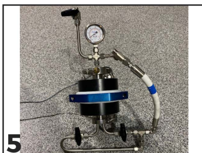
5 Best Practice: Set up an extraction adapter bypass (that can be quickly actuated through 3 way valves), a vent, and a pressure gauge.
