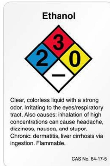
Figure 14 : Sample Ethanol NFPA 704 Hazard Rating Placard
